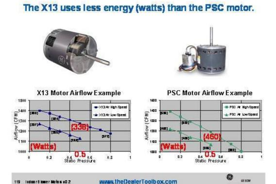
The ability to program the torque value by demand allows the HVAC manufacturer to deliver more precise airflow and only program the amount of selections needed..
